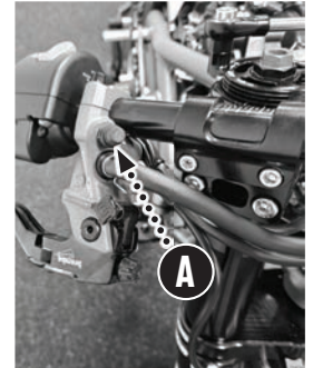
Front Brake Lever Bleed Screw (R Model)
