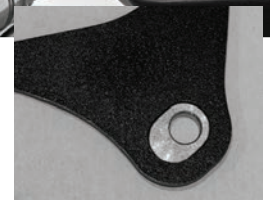
Suspension linkage plate with pull rod adjustment insert
