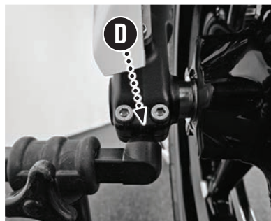
Positioning of two-pin Stand
