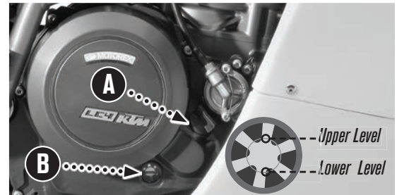
Oil Filler and Oil Window (R.H. side of engine)
