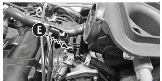
Fuel Rail Connector Screw
