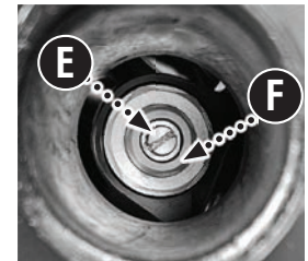
Compression Damping Adjuster Screw (Low and High Speed)
