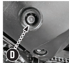
Compression Damping Adjuster Screw (Low and High Speed)
