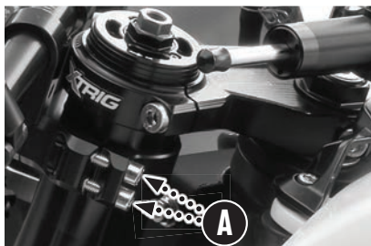
Handlebar Height and Angle Adjustment
