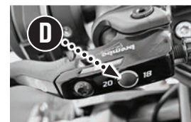
Front Braking Lever Ratio Adjustment Screw
