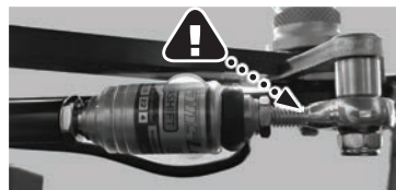
Quickshift Lever Adjustment (R Model)
