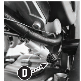
Fuel Pump Connector (unplugged)
